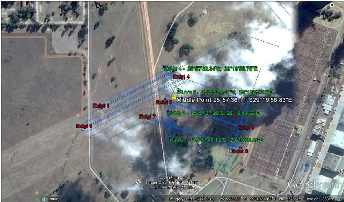
The Duvha By-Pass line is approximately 260m with 4 towers that are impacting on a watercourse. Please see image above for the tower footing coordinates, as well as the middle point of the activity.
